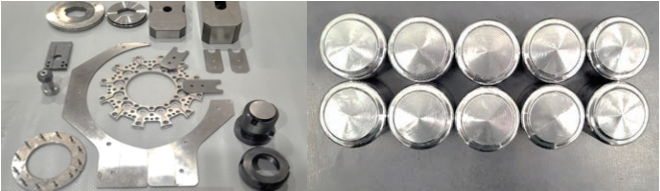
Tools (left) and dies (right) prepared by MyMint for coin production
